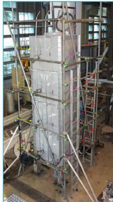
Figure 2: Erected SgTank FRP water storage tank system with locations of transducer points.
